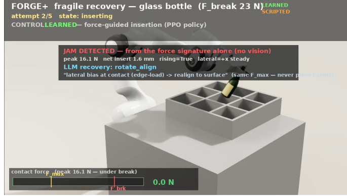
Figure 2: The rendered fragile recovery episode (Franka, glass-class bottle, F_{\text{break}} \approx 23\text{ N} ). The JAM card shows the actual signature the LLM saw — peak 16.1 N, net insert 1.6 mm, rising, lateral bias +x steady — its rotate_align decision, and the standing constraints: from the force signature alone (no vision) ; same F_{\text{max}} — never press harder .
