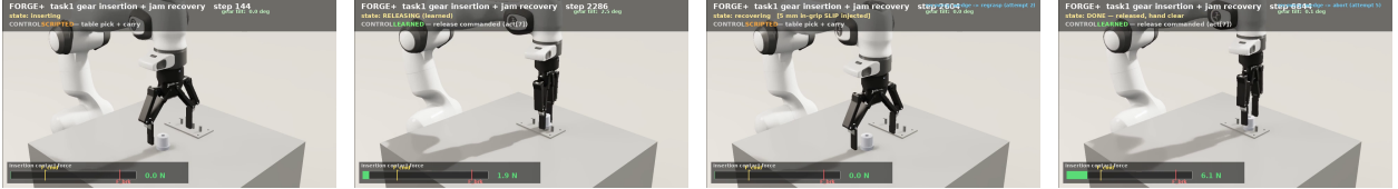
Figure 3: Stills from the released 2F-140 videos (HUD labels every phase LEARNED/SCRIPTED with a live force gauge vs. F_{\text{max}} and F_{\text{break}} ). Left to right: the scripted-staging table pick (a real friction grasp of the resting gear); the learned release firing at 1.9 N after a clean insertion; a recovery episode mid- regrasp — the tilted gear has been placed back on the table for a physical re-pick (LLM decision wedge → regrasp , attempt 2); the same episode ending seated, released, hand clear after two full regrasp cycles.
